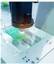
Surface inspection systems are having to meet increasing quality demands. Deviations in the structure, material defects and other issues must be detected quickly and reliably. This is where the strengths of embedded vision systems from Photonfocus come into play: They create images with the highest level of detail and deliver instant results thanks to onboard interpretation.
