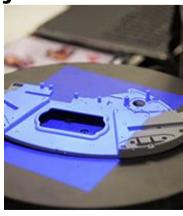
Complex components in the manufacturing industry are often made up of multiple geometries. Three-dimensional inspection systems are therefore needed to detect even the smallest deviations in production, so that they can be corrected. Embedded vision systems from Photonfocus are ideal for this task, combining different analysis methods to evaluate and interpret image data onboard.
